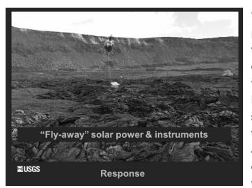
We also had the summit particularly we started to deploy these fly-away systems where we get our whole power assembly with solar panels that things was built up off site, off the monitoring site, and then helicoptered into these remote, fairly dangerous minimize areas to human exposure while they're hooking things up. This was our seismic
