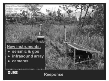
Our response also included deploy new instruments. We have of а cache undeployed instruments and we started to move things into this area to try to watch this seismicity and inflation. We had seismic and GPS instruments going in there almost immediately; infrasound array, there were two that were set up in the area. And then we installed a
